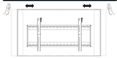
Push the display to left or right to enable fast alignment.
