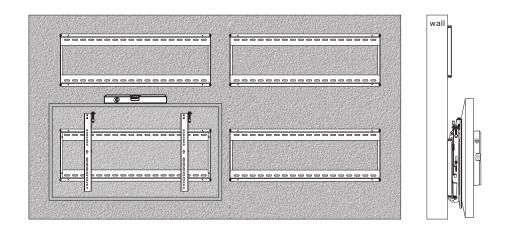
Adjust the display to keep level in vertical and horizontal directions.
