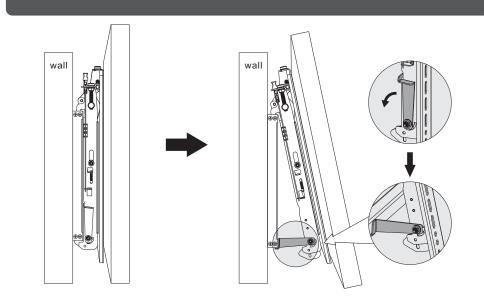
Kickstands provide tilt access for easy cables management and maintenance.
