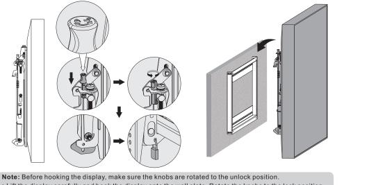
· Lift the display carefully and hook the display onto the wall plate. Rotate the knobs to the lock position for secure the display.
